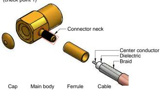
Step 2. Please slide ferrule onto cable and splay out cable braid
